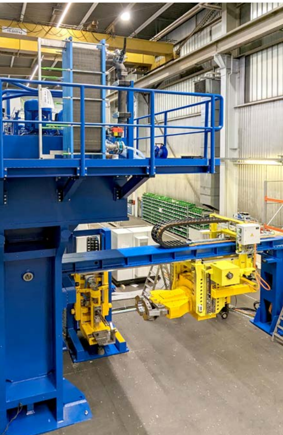
The hydraulic direct drive of the VPE multi-purpose press enables up to 120 strokes per minute.
