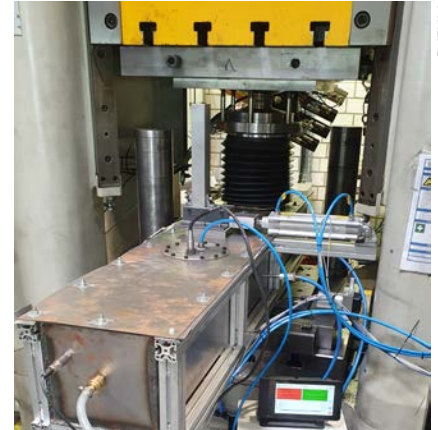
The tool enclosure for low-oxygen forging during tests at IFUM (Hannover).
